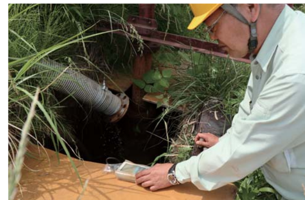
Contact of rainwater seeping underground with ore may generate acid water containing heavy metals. Therefore, it is necessary to monitor water from surrounding springs even at suspended and closed mines continually.
